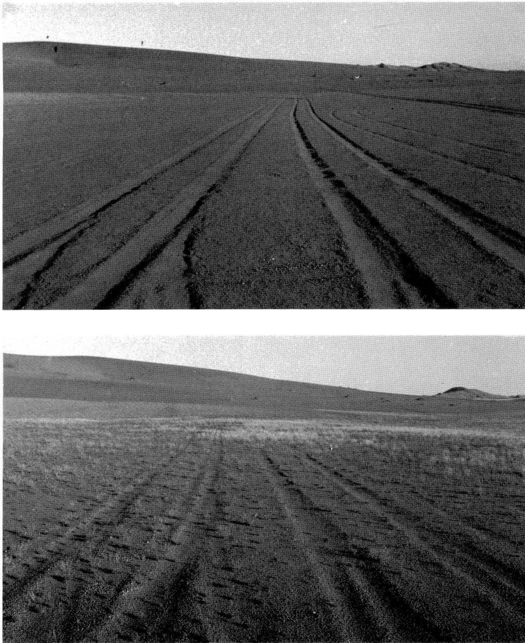
Fig. 3 (a) Tracks on gravel-covered sand photographed on day tracks were made, following afternoon wind. The tracks on the left were made by the Land Rover driving in the same track ten times, while those on the
